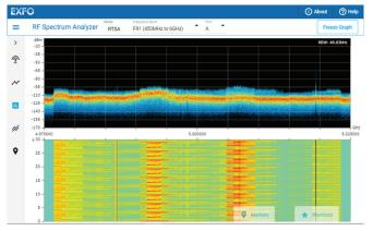
Figure 1. Real-time persistence spectrum and spectrogram.
