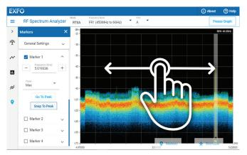
Figure 2. Patent pending Snap-to-Peak feature.
